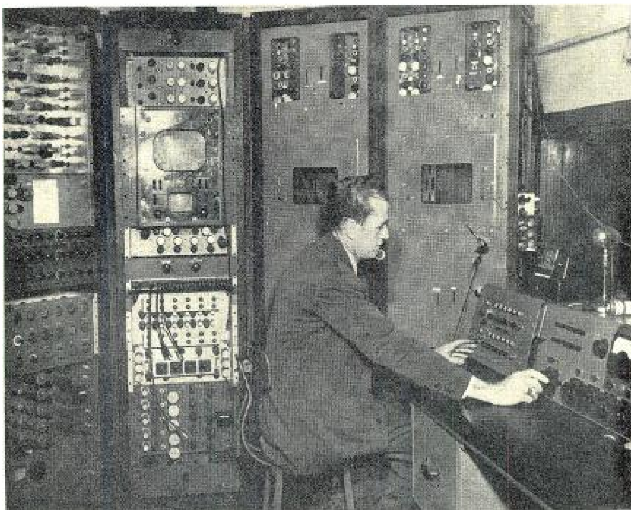
Fig. 3 — Experimental color television equipment installed in the control room of the Wardman Park studio.
