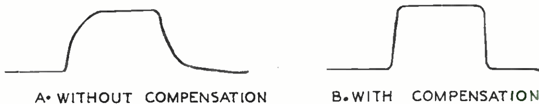
Fig. 27 — Waveforms resulting from the scanning of a white bar on a black background in a flying-spot scanner, showing the effect of phosphor decay time.
